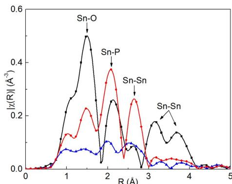
**Black:** Crystal structure of Sn<sub>4</sub>P<sub>3</sub>; High Sn-O peak is from particle surfaces or an amorphous oxide phase;
