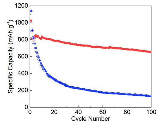
The Sn<sub>4</sub>P<sub>3</sub>/graphite composite (red) exhibits excellent electrochemical performance compared to pure Sn<sub>4</sub>P<sub>3</sub> (blue), with a reversible capacity of 651 mAh/g in the 100th cycle.
