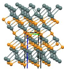
Sn<sub>4</sub>P<sub>3</sub> is a promising conversion-type anode material for LIB with a theoretical capacity of 1255 mAh/g.
