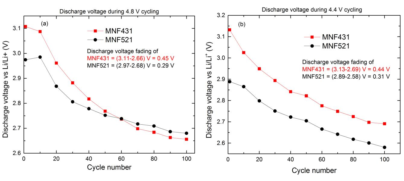
Comparison of equilibrium discharge voltage vs cycle number of MNF521 and MNF431 cathodes at 4.8 V (a) and 4.4 V (b) cut off voltage.
