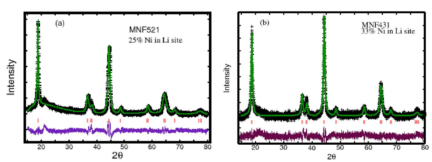
GSAS fitting showed more cation mixing in Ni rich material with 33% of Ni in Li sites in MNF 431 (b) and 25% in MNF521 (a) in agreement with the intensity ratio from modelling the cation disorder in Li layered oxide LiNiO<sub>2</sub> (CrystalMaker software). The ratio of I(003)/I(104) decreases with increasing the cation mixing.
