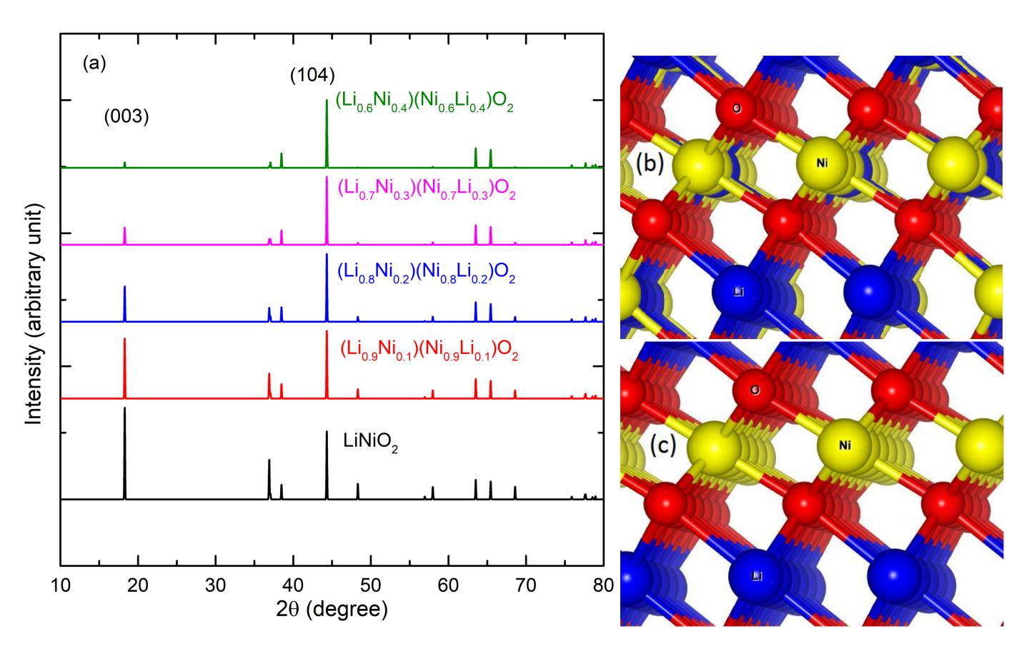
XRD modeling (CrystalMaker software) of Li and Ni mixing (a), structural visualization of cation mixing (b), ideal crystal structural of layered LiNiO<sub>2</sub> (c)
