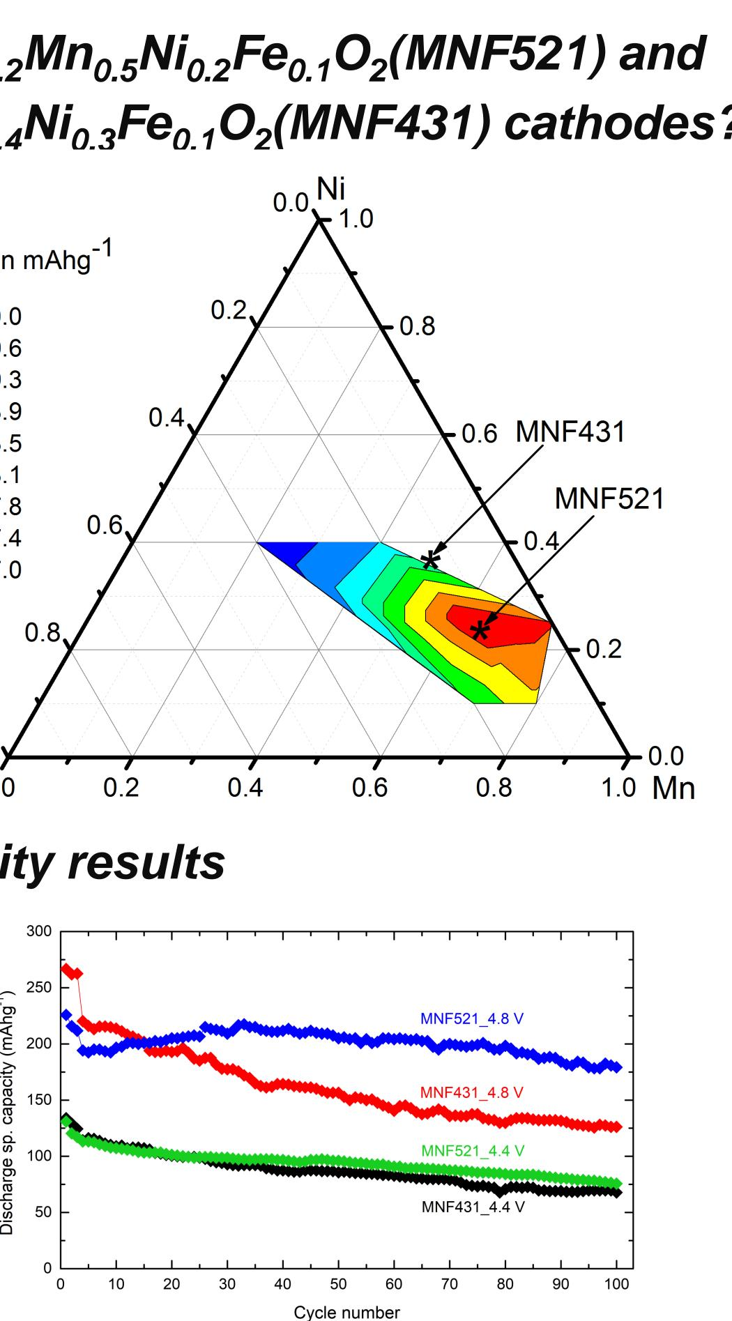
Cycling of MNF521 and MNF431 at different cut off voltages. First 3 cycles at 0.1C and all other cycles at 0.3C, C = 250mAhg<sup>-1</sup>.
