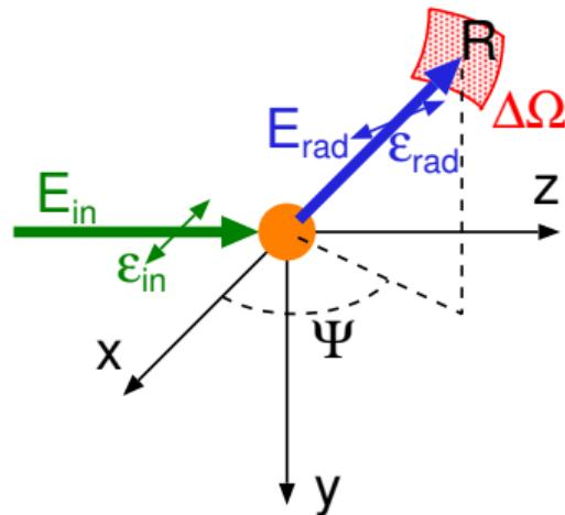
$$\frac{d\sigma}{d\Omega} = \frac{|E_{rad}|^2}{|E_{in}|^2} R^2 = r_0^2 \sin^2 \Psi$$
