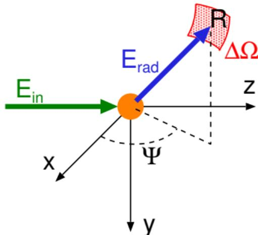
detector of solid angle  $\Delta\Omega$  located a distance  $R$  from electron
