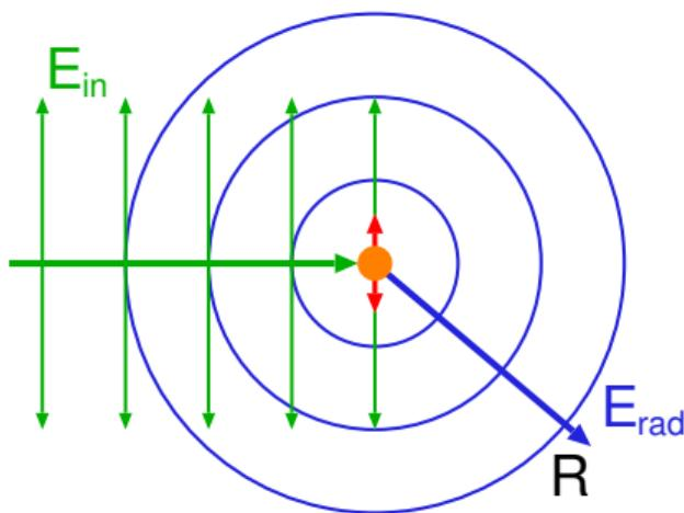
The electron is exposed to the incident electric field  $E_{in}(t')$  and is accelerated
