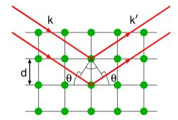
The Bragg condition for diffraction is derived by assuming specular reflection from parallel planes separated by a distance d.
