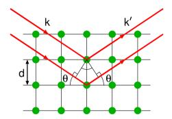
The Bragg condition for diffraction is derived by assuming specular reflection from parallel planes separated by a distance d.
