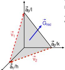
The plane with Miller indices (hkl) intersects the three basis vectors of the lattice at  $a_1/h$ ,  $a_2/k$ , and  $a_3/l$
