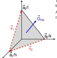
The plane with Miller indices (hkl) intersects the three basis vectors of the lattice at  $a_1/h$ ,  $a_2/k$ , and  $a_3/l$
