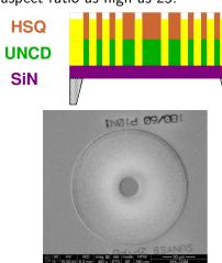
Making high aspect ratio zone plates is challenging but a new process has been developed to make plates with an aspect ratio as high as 25.
