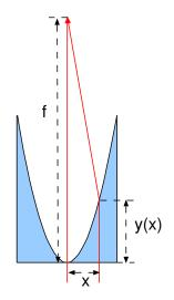
In calculating the optimal surface profile for a refractive lens, an important approximation was made which resulted in a parabolic surface
