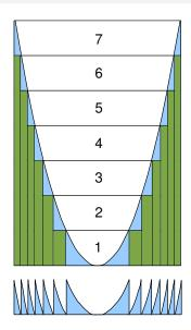
The outermost zones become very small and thus limit the overall aperture of the zone plate. The dimensions of outermost zone, *N* can be calculated by first defining a scaled height and lateral dimension
