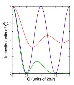
Previously we derived the scattering intensity from two localized electrons both fixed and randomly oriented to the x-rays
