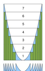
The outermost zones become very small and thus limit the overall aperture of the zone plate. The dimensions of outermost zone, *N* can be calculated by first defining a scaled height and lateral dimension
