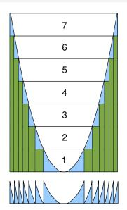
The outermost zones become very small and thus limit the overall aperture of the zone plate. The dimensions of outermost zone, *N* can be calculated by first defining a scaled height and lateral dimension
