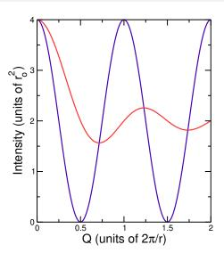
Previously we derived the scattering intensity from two localized electrons both fixed and randomly oriented to the x-rays
