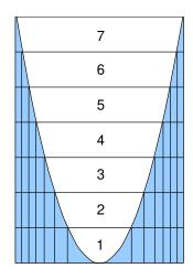
Mark off the longitudinal zones (of thickness  $\Lambda$ ) where the waves inside and outside the material are in phase.
