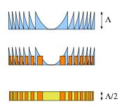
The specific shape required for a zone plate is difficult to fabricate, consequently, it is convenient to approximate the nearly triangular zones with a rectangular profile.
