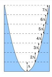
Mark off the longitudinal zones (of thickness  $\Lambda$ ) where the waves inside and outside the material are in phase.
