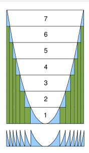
Mark off the longitudinal zones (of thickness  $\Lambda$ ) where the waves inside and outside the material are in phase.
