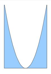
The ideal refracting lens has an elliptical shape but this is impractical to make. Assuming the parabolic approximation:
