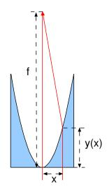
In calculating the optimal surface profile for a refractive lens, an important approximation was made which resulted in a parabolic surface
