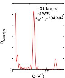
This combines the Kiessig fringes from the entire multilayer and the interference obtained because of the bilayer repetition
