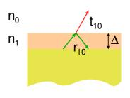
$r_{01}$  - reflection in  $n_0$  off  $n_1$  $t_{01}$  - transmission from  $n_0$  into  $n_1$
