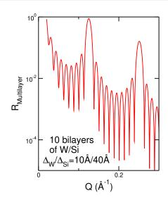
Using the kinematical approximation, we have calculated the reflectivity of a multilayer of slabs containing two contrasting elements
