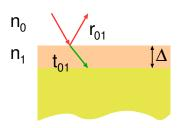
$r_{01}$  - reflection in  $n_0$  off  $n_1$  $t_{01}$  - transmission from  $n_0$  into  $n_1$
