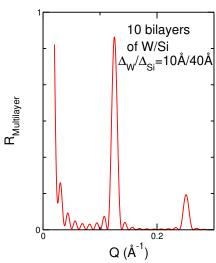
Using the kinematical approximation, we have calculated the reflectivity of a multilayer of slabs containing two contrasting elements
