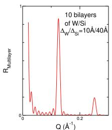
This combines the Kiessig fringes from the entire multilayer and the interference obtained because of the bilayer repetition
