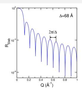
Recall the reflection coefficient for a thin slab.
