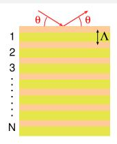
N repetitions of a bilayer of thickness  $\Lambda$  composed of two materials, A and B which have a density contrast  $(\rho_A > \rho_B)$ .
