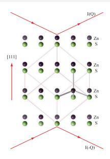
The ZnS structure is not centrosymmetric and when viewed along the  $\langle 111 \rangle$  direction, it shows alternating stacked planes of Zn and S atoms.
