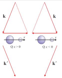
Two unlike atoms with scattering factors  $f_1$  and  $f_2$  are oriented by a vector pointing from the larger to the smaller.
