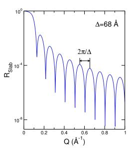
Recall the reflection coefficient for a thin slab.
