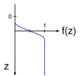
Since most interfaces are not sharp, it is important to be able to model a graded interface, where the density, and therefore the index of refraction varies near the interface itself.
