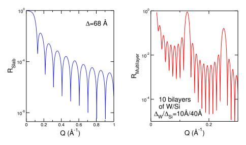
Treat the multilayer as a stratified medium on top of an infinitely thick substrate.
