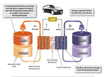
$During\ discharge,\ electrons\ are\ moving\ through\ the\ circuit,\ while\ Li\ ions\ are\ moving\ through\ the\ ion\ exhange\ membrane\ to\ the\ opposite\ electrode.\ During\ charge,\ the\ processes\ are\ reversed.$
