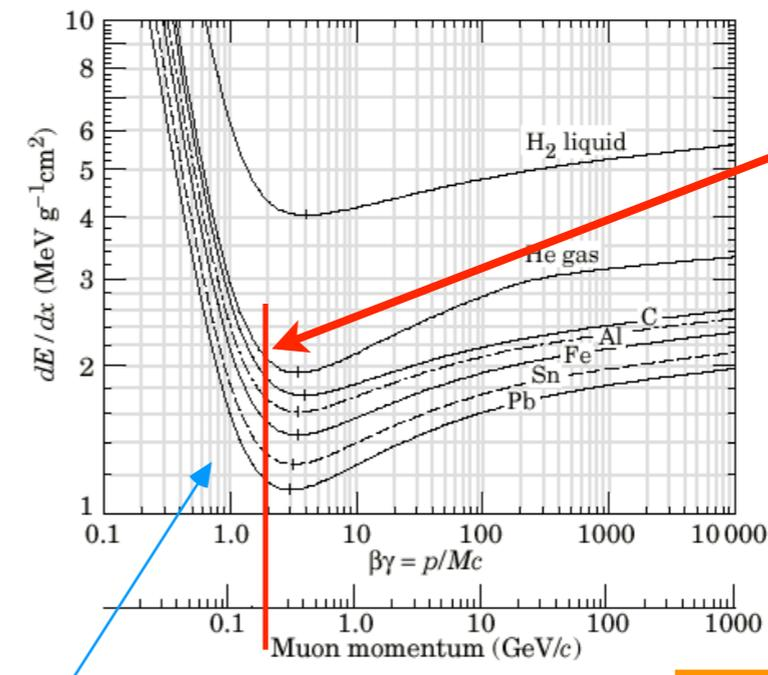
● optimal working point is  $\approx$  ionization minimum
